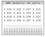
The BMS Details page shows all individual cell voltages, plus a bar graph below. Dotted lines on the graph show HV and LV thresholds plus hysteresis.
