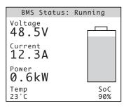
The BMS Status page is the standard display when the system is running, showing pack voltage, current, power, temperature, battery state of charge. This will only be shown if a current sensor is present.
