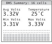
The BMS Summary page shows the average, minimum and maximum cell voltages, and the temperature sensor, plus a bar graph overview of all cells across the bottom.
